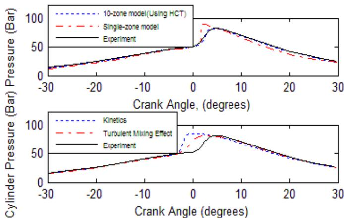
Figure 6. Comparison between single and multi-zone model [51].
