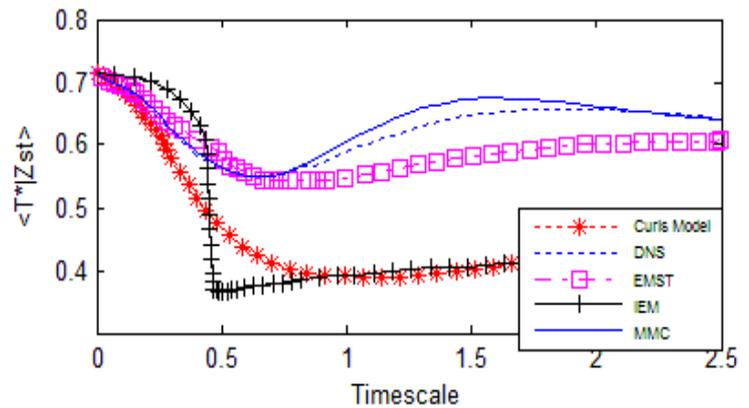
Figure 7. Stoichiometric temperature results for various mixing models [57,58]
