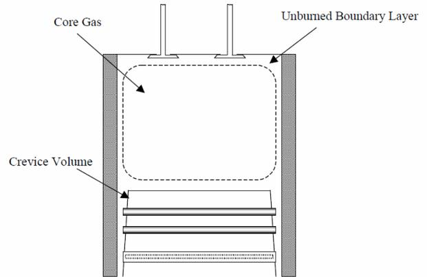
Figure 4. General layout of the quasi-dimensional simulation showing the interacting adiabatic core, thermal boundary layer and crevice regions [48].
