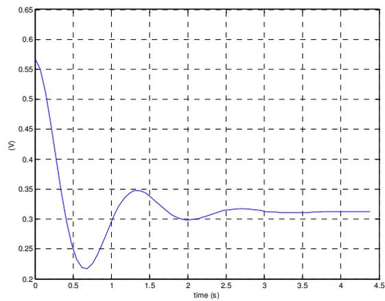
**Figure 6: Simulated Transient Response of PI Controller Output**
