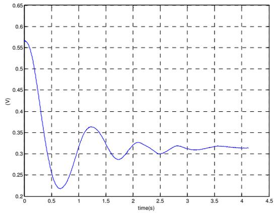
**Figure 5: Measured Transient Response of PI Controller Output**
