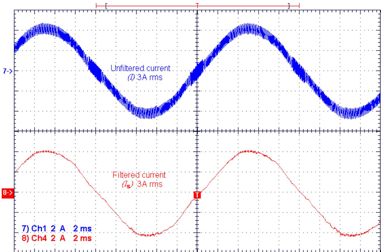
Figure 3: Inverter Output Current Waveform ( $I_{ref} = 3A$ )
