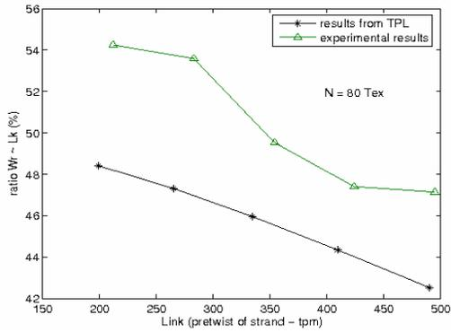
**Fig. 4.** The relationship between twist of strand and helix twist angle of a plied yarn: comparison between experimental results and the results from the present work using strands of 80 Tex.
