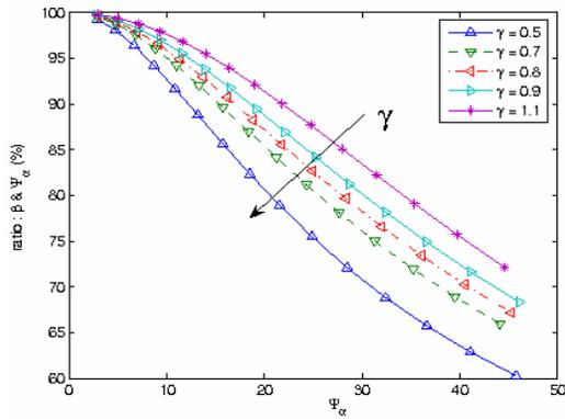
**Fig. 2.** Relationship between the twist angle of strand and helix twist angle of balance plied yarn using different  $\gamma$ 's
