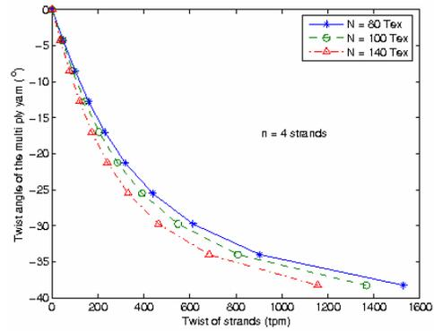
**Fig. 5.** The relationship between twist of strands and helix twist angle of a multi ply yarn for the different cases of used yarn counts : 80, Tex 100 Tex and 140 Tex using 4 strands.
