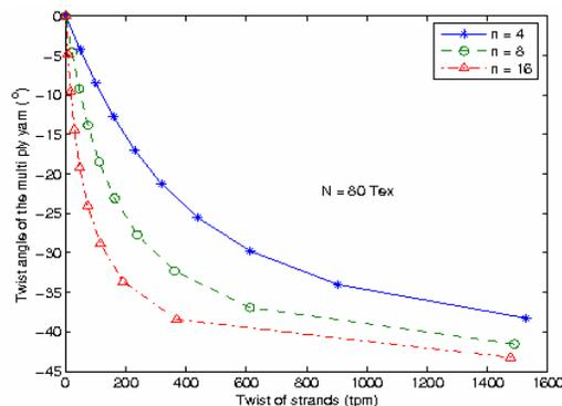
**Fig. 6.** Relationship between twist of strands and helix twist angle of plied yarn for the cases of 4, 8, 16 strands of 80 Tex
