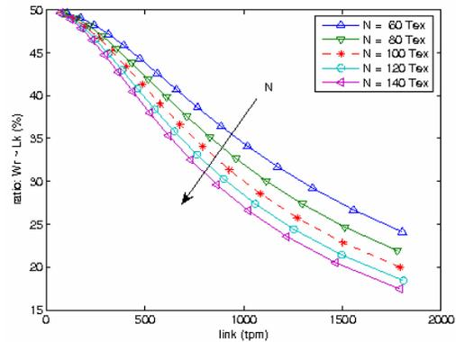
**Fig. 3.** Relationship between the twist angle of strand and helix twist angle of a balance plied yarn using different yarn counts
