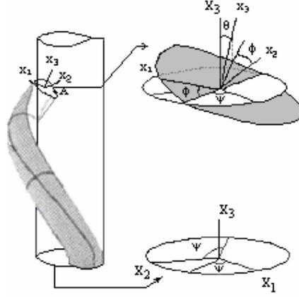
**Fig. 1** Schema of a strand ( $r$ ) wound on a cylinder ( $R$ ): the fixed cartesian and moving coordinate frames.
