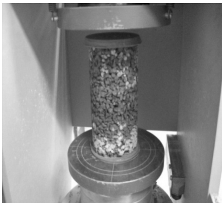
Figure 2. Compressive strength testing rig
