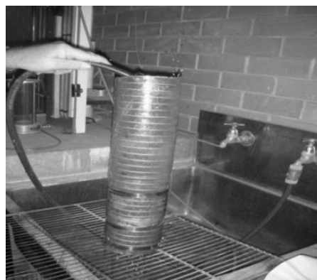
Figure 3. Permeability testing rig
