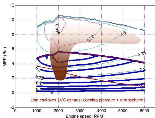
**Figure 2: Modeled operating efficiencies for a two position VCR engine. The lower set of contours (thick blue lines) peak at above 35% at a little over 2,000 rpm and produce about 5 Bar MEP. This equates to about 17 kW engine output power for a 2 litre engine.**
