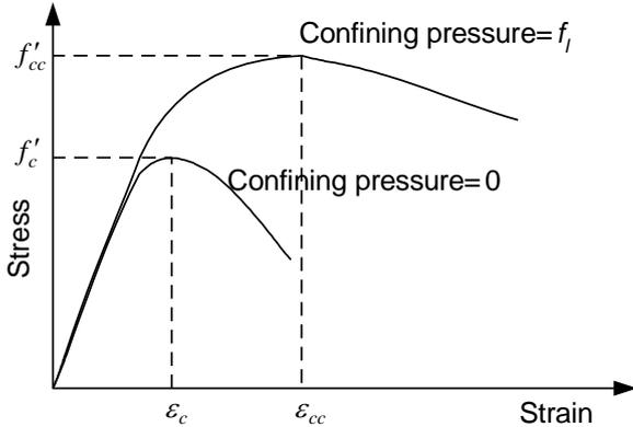
Figure 1. Typical stress-strain relationship for confined and unconfined concrete.
