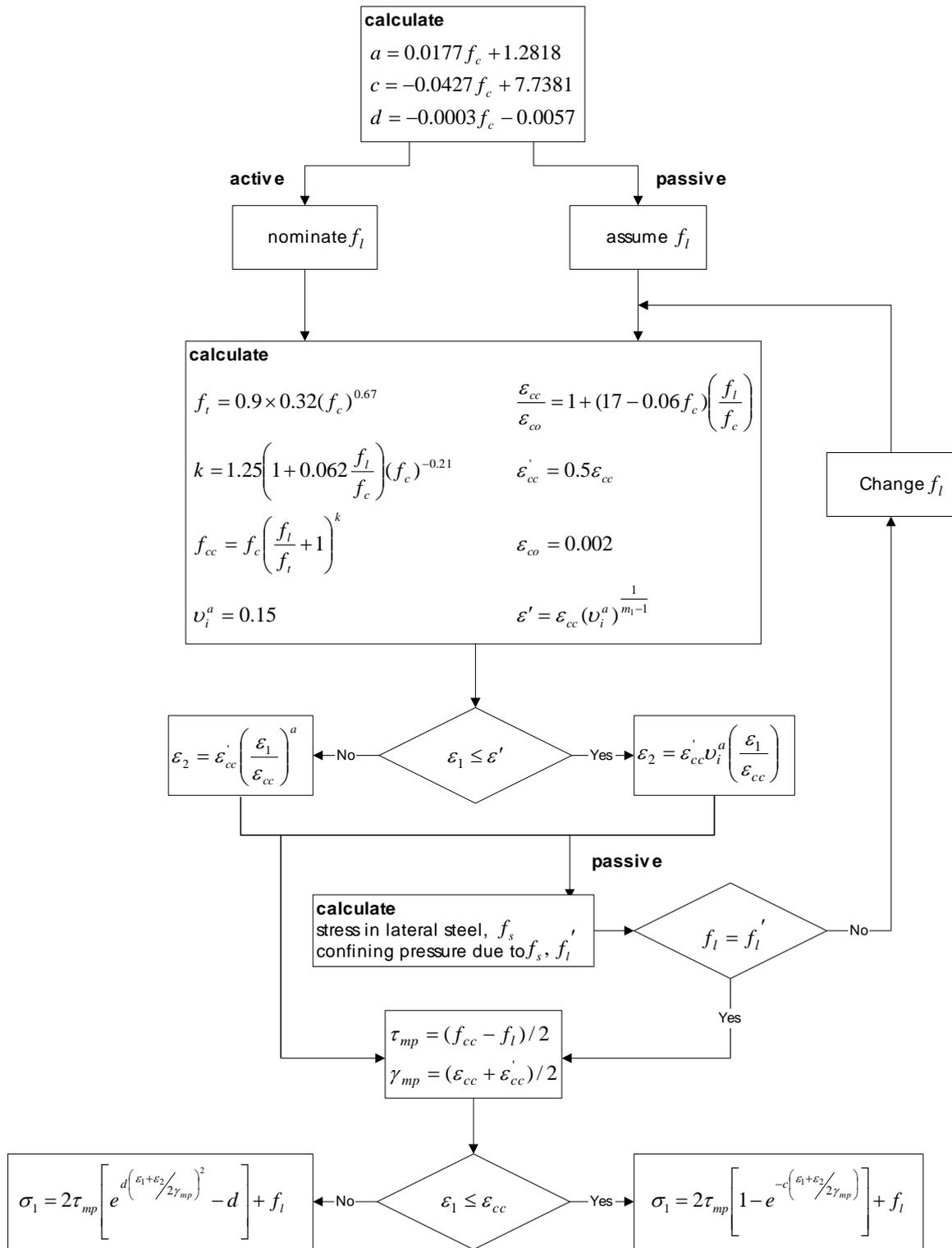
Figure 3. Procedure in drawing stress-strain curves for confined concrete.
