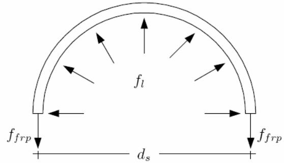
Figure 2. Confinement action in FRP composites.
