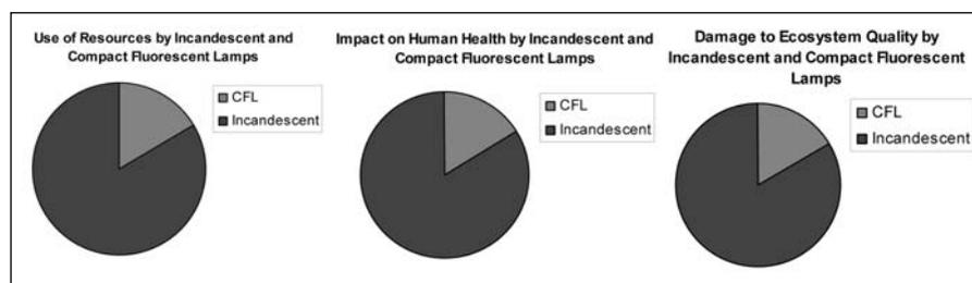
Figure 4. Comparisons of incandescent and compact fluorescent lamps for environmental damage categories of Use of resources (MJ surplus energy), Impact on human health (DALY) and Damage to ecosystems (PDF\*m<sup>2</sup>yr).
