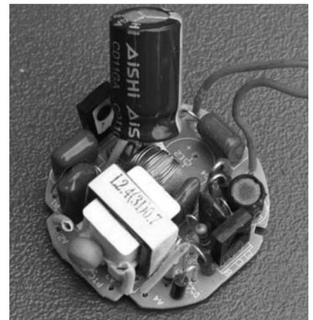
Figure 6. The ballast circuit of the compact fluorescent lamp.
