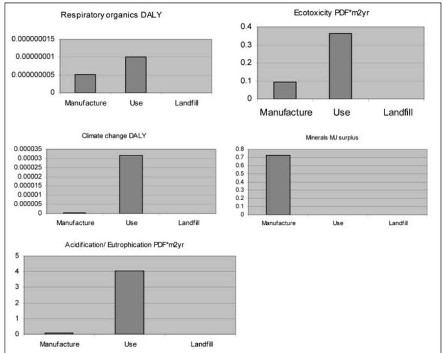
Figure 5. Relative impact on various criteria of stages of life of a compact fluorescent lamp.
