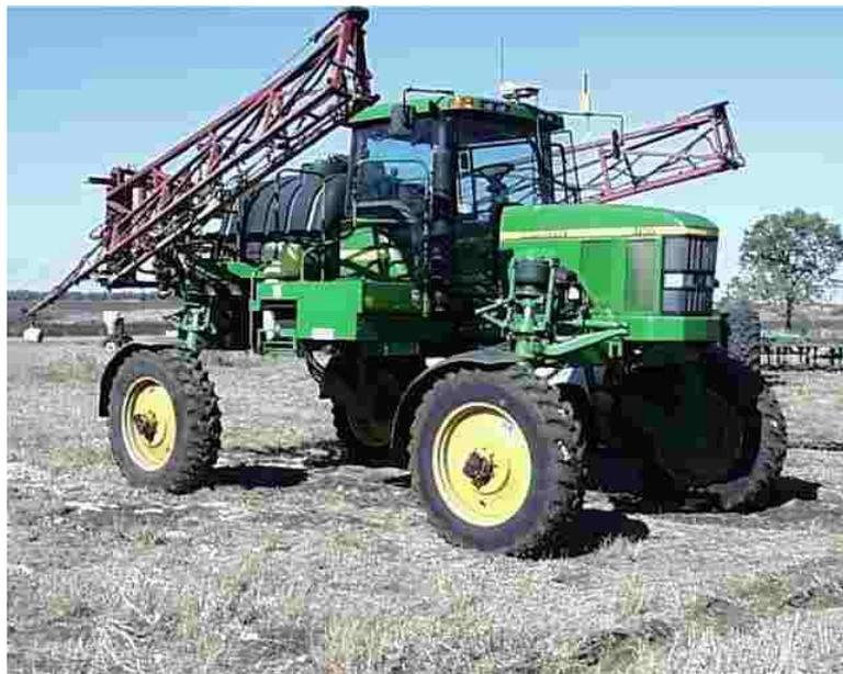
**Figure 1:** GPS and Radio Antennae on Spray Rig
