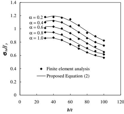
Figure 3. Ultimate strengths of steel plates
