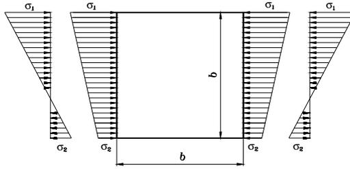
**Figure 1. Clamped steel plates under edge compression and in-plane bending**
