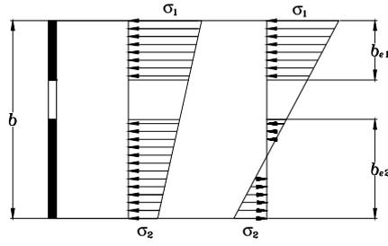
Figure 5. Effective width of steel plate under compression and in-plane bending
