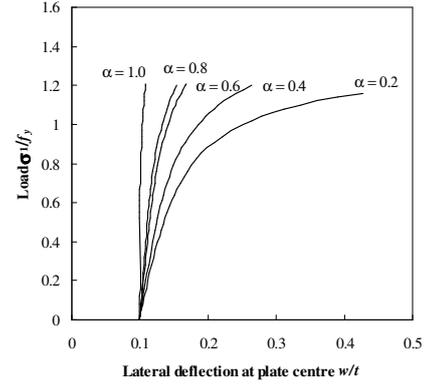
Figure 4. Steel plates under in-plane bending
