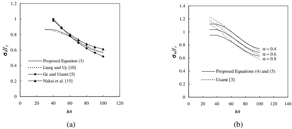
Figure 6. Comparison of the proposed formulas with those presented by other researchers: (a) uniform compression; (b) Non-uniform compression
