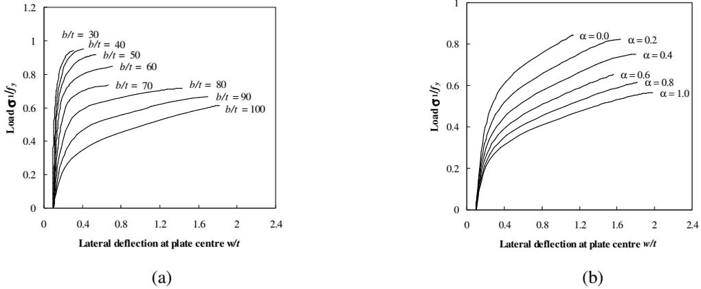
**Figure 2. Load-deflection curves for steel plates under stress gradients: (a)  $\alpha = 0.8$  ; (b)  $b/t = 100$ .**
