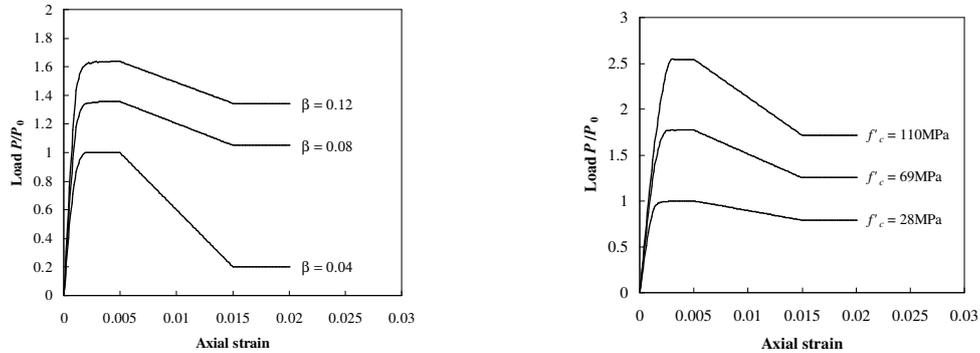
Figure 4. Behavior of CFST columns: (a) effects of steel ratios; (b) effects of concrete strengths
