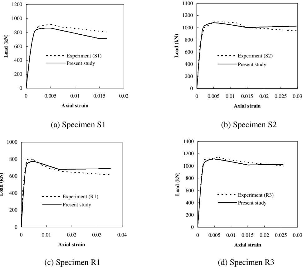
Figure 3. Comparison of present study with experimental results
