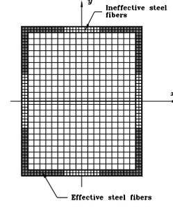
Figure 2. Effective fibers in CFST section
