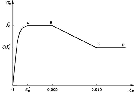
Figure 1. Stress-strain curve for concrete
