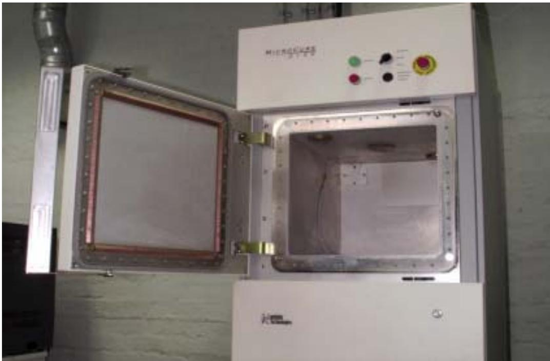
**Figure 10: Cavity of Microcure 2100 model 250**
