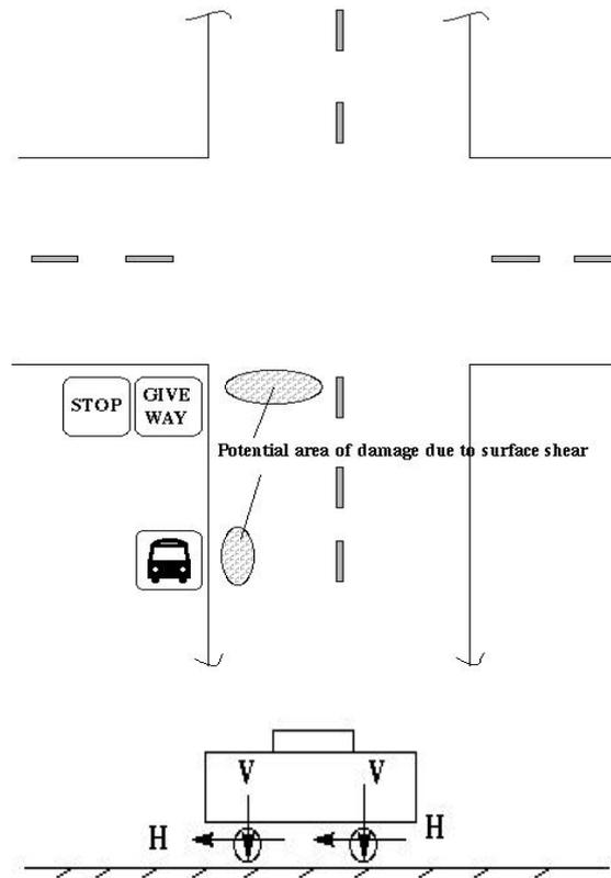
**Figure 1: Potential failures of road pavement due to surface shear.**
