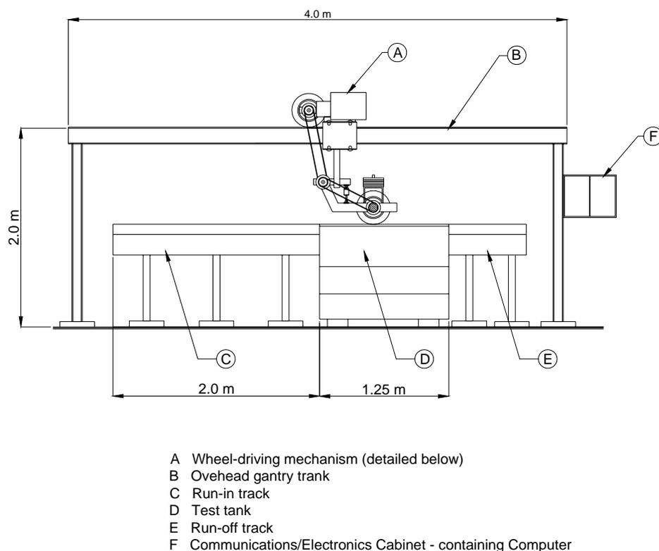
**Figure 5: A conceptual diagram showing the testing rig.**
