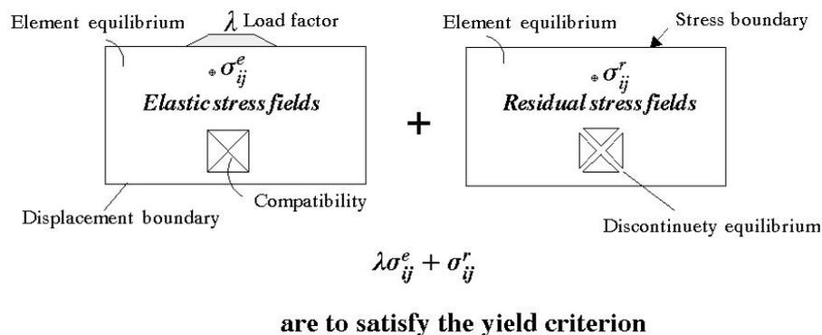
**Figure 3: Finite element application of Melan's static shakedown theorem.**
