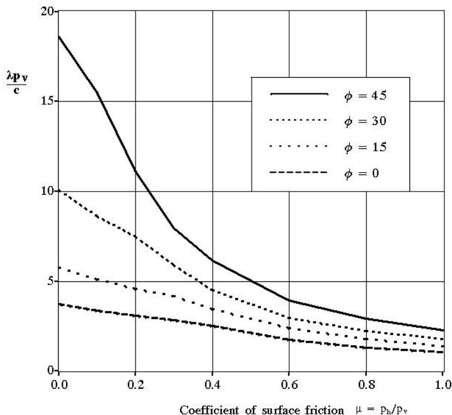
**Figure 4: Effect of coefficient of surface friction upon dimensionless shakedown limits for various soil frictional angles.**
