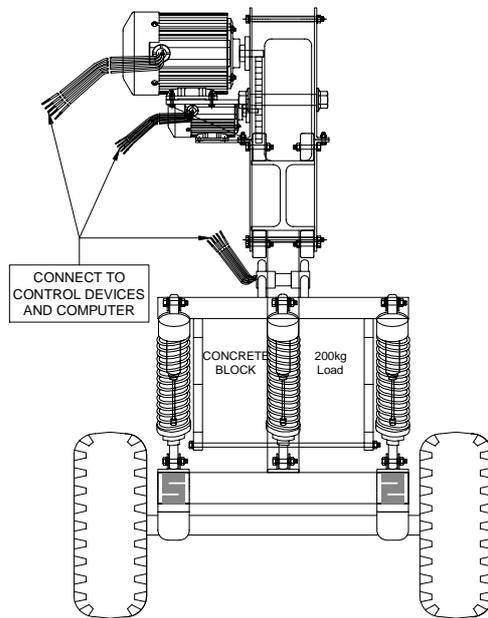
**Figure 6: Initial design of the driving mechanism.**
