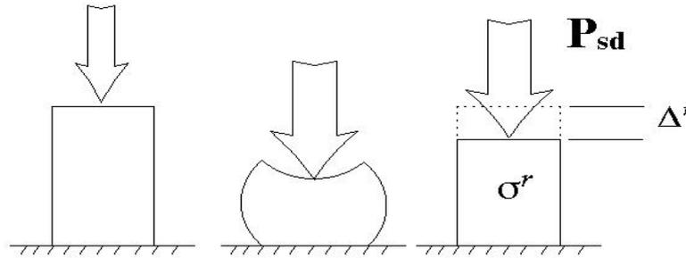
**Figure 2: Simple illustration of shakedown concept.**
