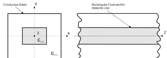
Fig. 1. Shielded dielectric rod waveguide.
