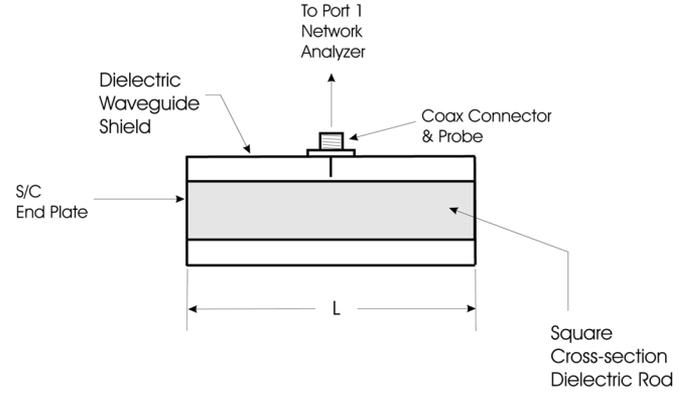
Fig. 7. Dielectric resonator used for the measurement of unloaded  $Q$ .
