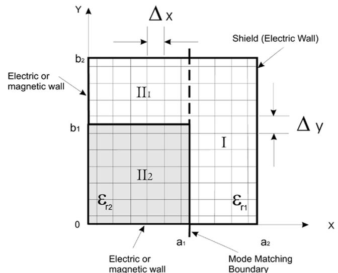
Fig. 2. One quadrant of the cross section showing the grid for power loss calculation.
