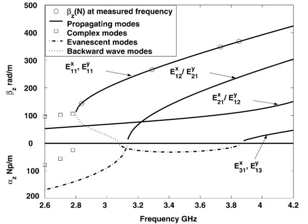
Fig. 9. Calculated propagation coefficient values for the first few modes to propagate, with measurements of the  $E_{11}^y$  mode superimposed. Shield dimension ratio SDR = 1.98..
