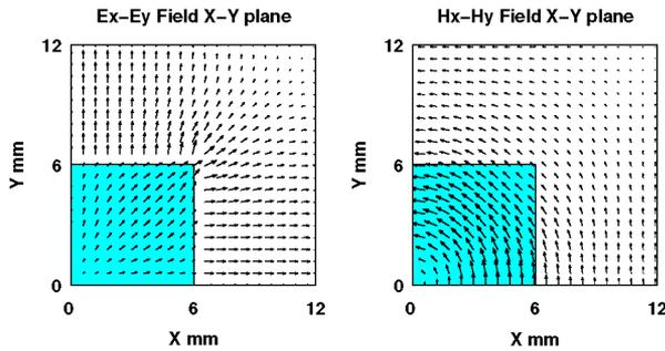
Fig. 6. Electric and magnetic field patterns in the  $xy$ -plane for the coupled  $E_{21}^x/E_{12}^y$  modes. For clarity, the electric field intensity in the dielectric is  $\times 5$ . (Color version available online at <http://ieeexplore.ieee.org>.)
