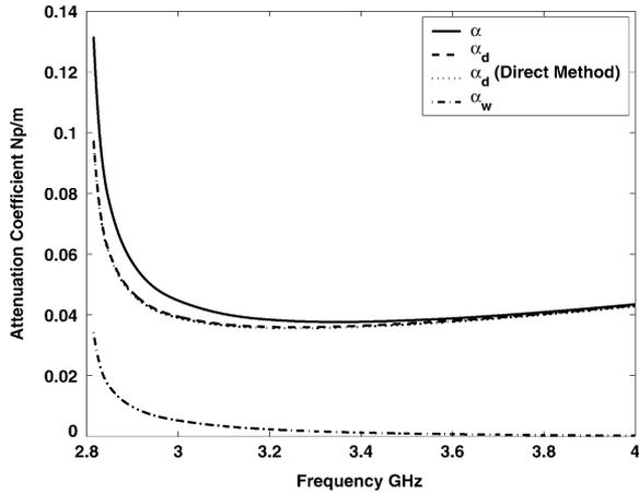
Fig. 3. Attenuation coefficient versus frequency for the  $E_{11}^y$  mode. The SDR is  $\text{SDR} = a_2/a_1 = 2$ .
