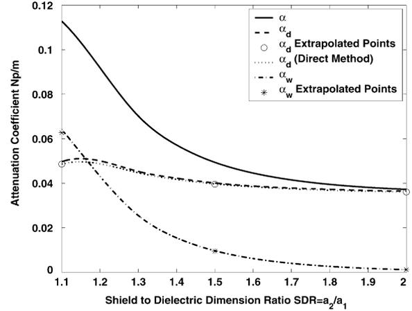
Fig. 4. Attenuation coefficient versus SDR for the  $E_{11}^y$  mode. The frequency is 3.4 GHz.
