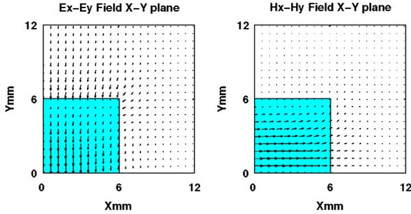
Fig. 5. Electric and magnetic field patterns in the  $xy$ -plane for the  $E_{11}^y$  mode. (Color version available online at <http://ieeexplore.ieee.org>.)
