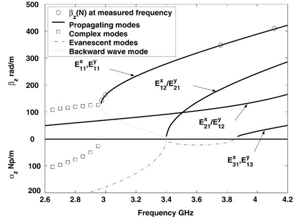
Fig. 8. Calculated propagation coefficient values for the first few modes to propagate, with measurements of the  $E_{11}^y$  mode superimposed. Shield dimension ratio SDR = 1.49.
