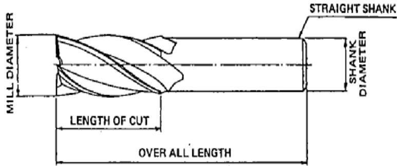
Figure 1: Straight Shank End mill
