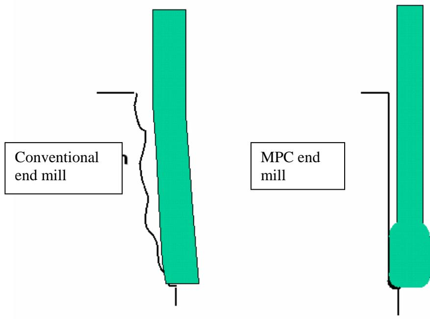
Figure 12: Comparison between MPC and conventional end mills
