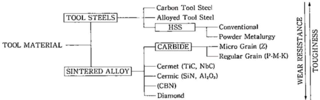
Figure 7: Various types of tool materials
