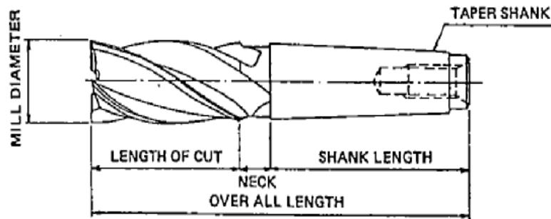
Figure 2: Taper Shank End mill
