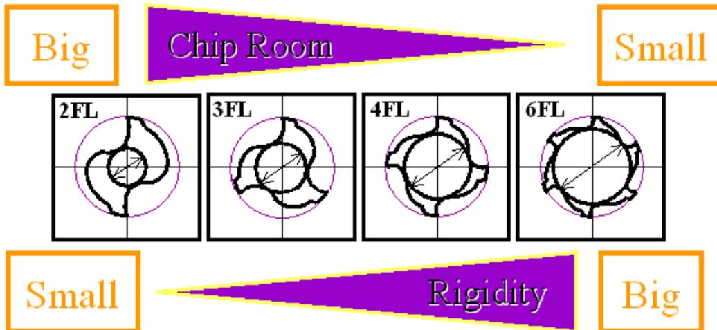
Figure 5: Chip Room and Rigidity of End Mills
