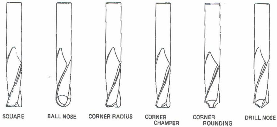
Figure 6: Various types of end profile in end mills
