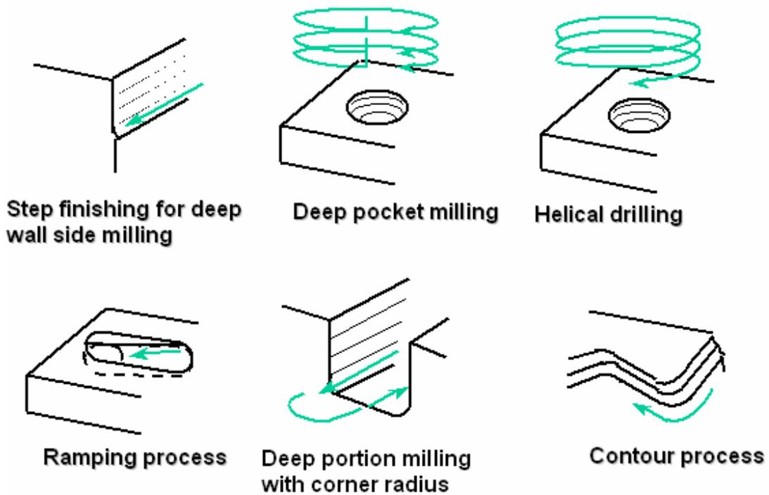
Figure 13: Various applications of MPC end mill
