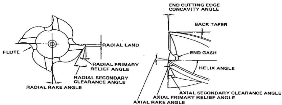
Figure 3: Terminology of an end mill
