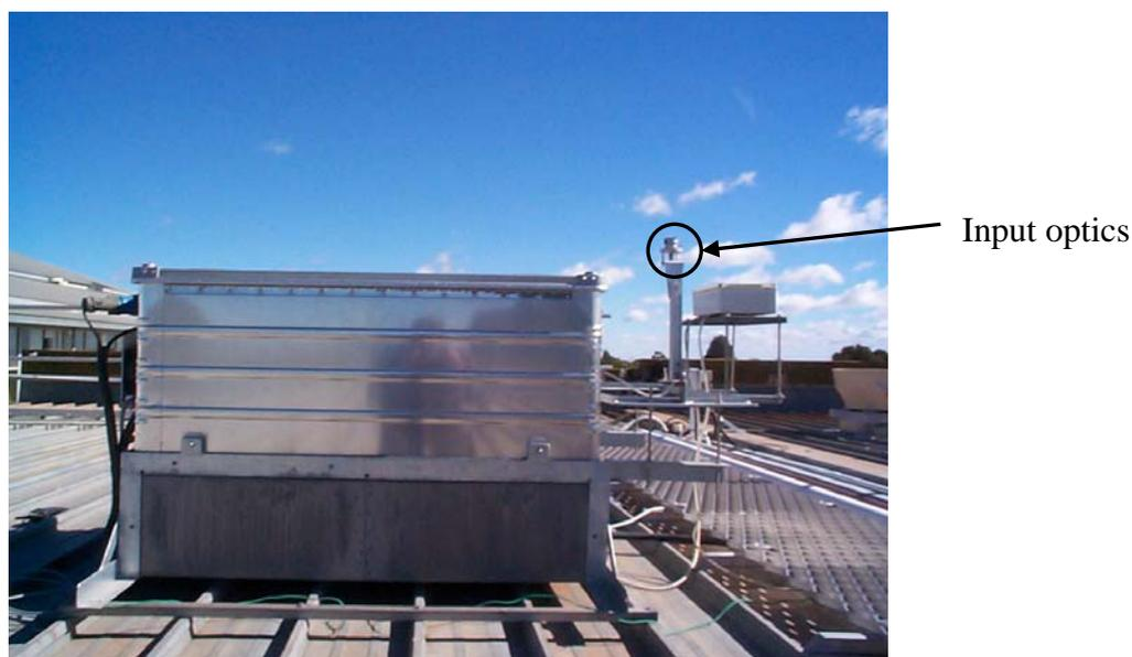
Figure 1: Automated solar UV spectroradiometer enclosed in the weatherproof container on an unshaded roof.
