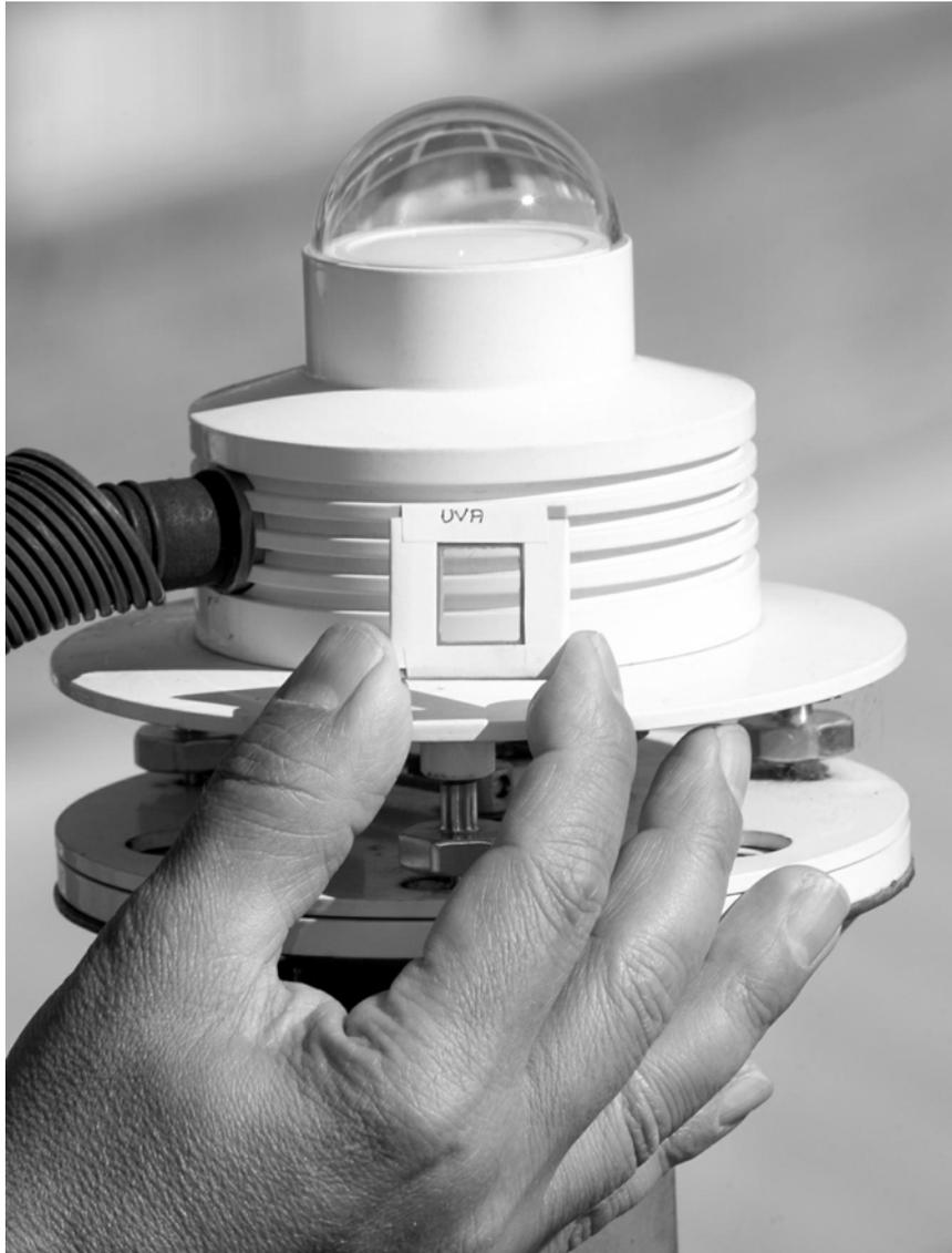
Figure 1 – The UVA dosimeter next to the UVA meter employed for the calibration of the dosimeters.
